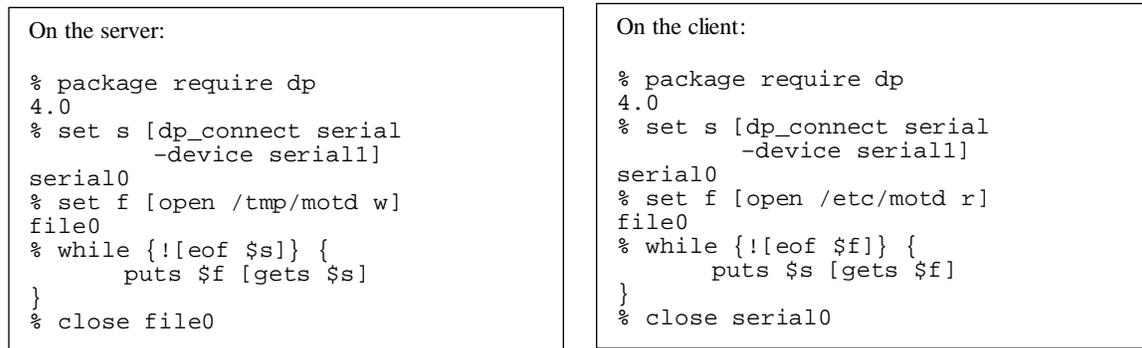
Figure 3 – Communication over a serial connection
